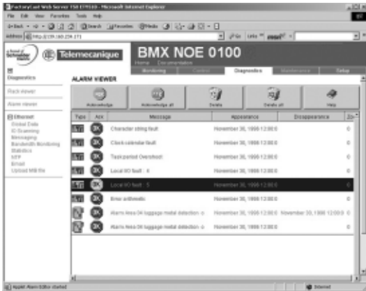
Alarm display from the diagnostic buffer
